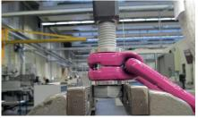
Pic. 5: Dismantling position of the L-VLBG
