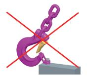
*Pic. 2: Use only suitable lashing means for hanging or hooking into the L-VLBG*
