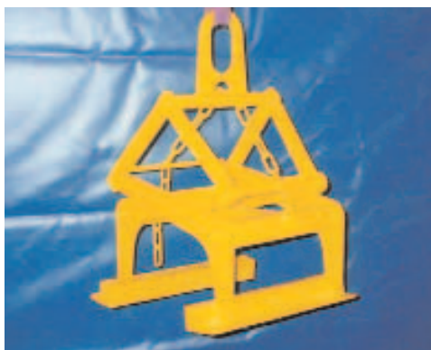
Garra Tipo BFZ concrete pices grab BFZ
